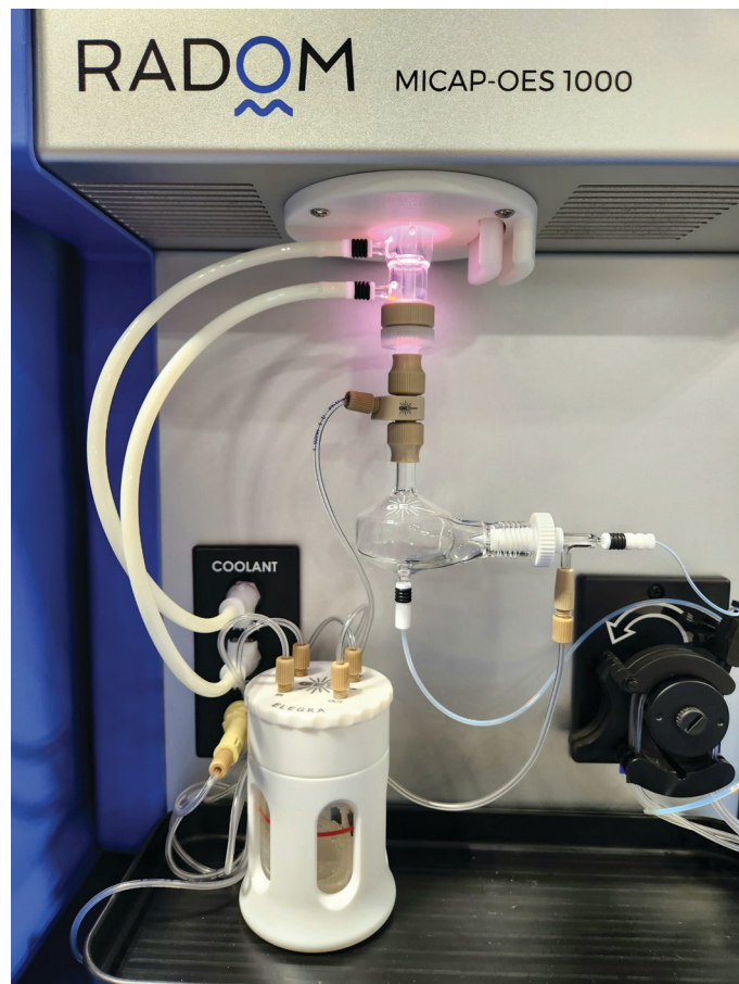
Figure 1. MICAP sample introduction area with Glass Expansion accessories utilized in this brine analysis
